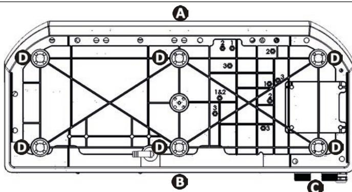
View of the appliance base from below for installing the anti-vibration blocks
