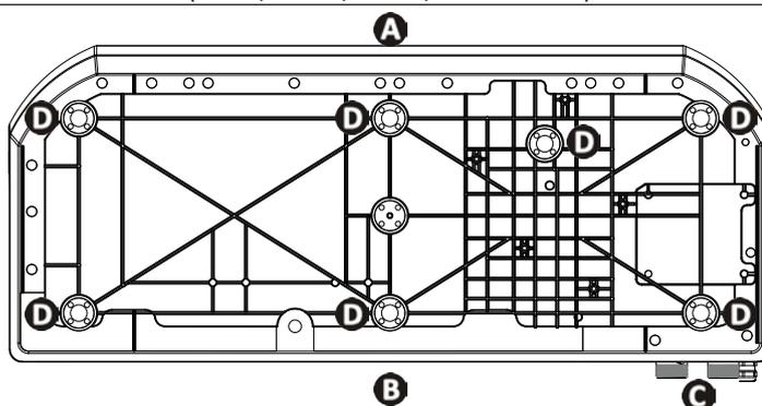
View of the appliance base from below for installing the anti-vibration blocks
