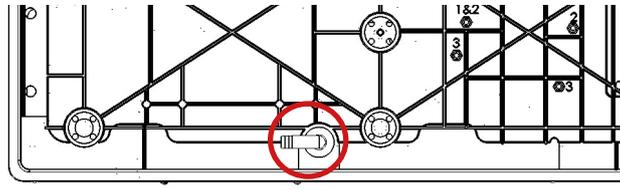
Condensate drainage elbow (view of the device from below)
